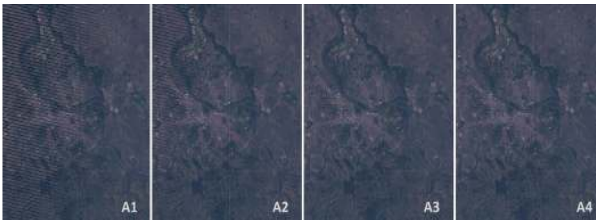
Figure 6. Focal Analysis gap removal. A1 SLC off image A2, A3 gap fill stage A4 Focal Analysis gap clean image
